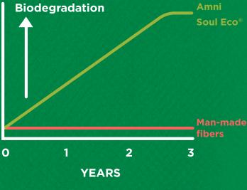
\*Based on ASTM D5511 - Standard Test Method for Determining Anaerobic Biodegradation of Plastic Materials Under High-Solids.
